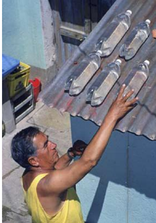
Figure 3: Clear plastic bottles full of raw water are placed on a corrugated iron sheet for disinfection by sunlight
